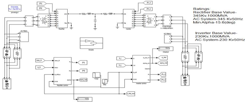
Fig 5. Simulink model of HVDC System
