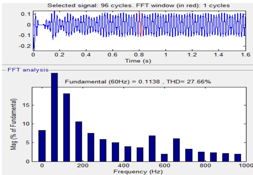
**Fig.18** THD Analysis for Inverter Current using PI controller
