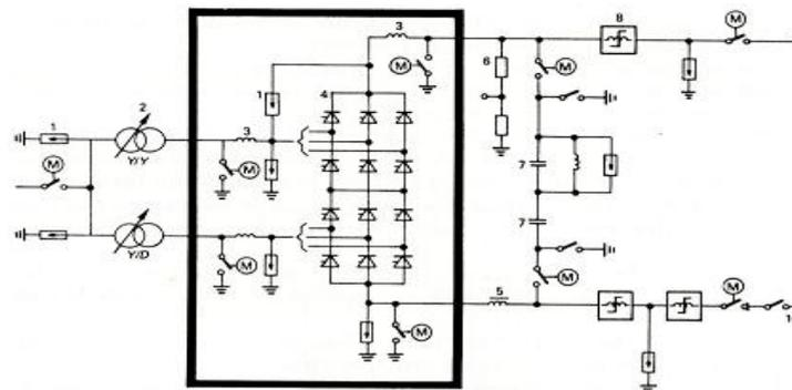
**Fig2 The Main Circuit Diagram for One Pole of a Converter Station.**
