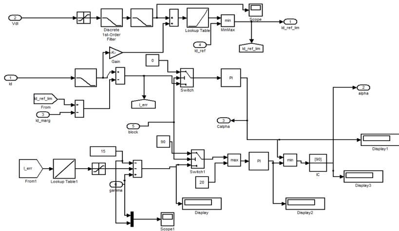
Fig 4. Inverter control with PI.
