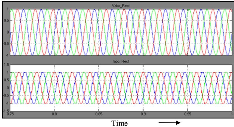
**Fig 6.** Rectifier side AC Voltage and AC Current
