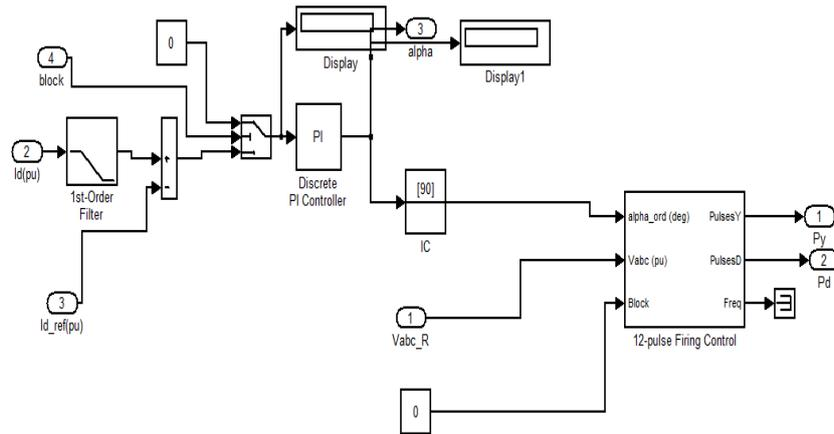
Fig 3. Rectifier control with PI.
