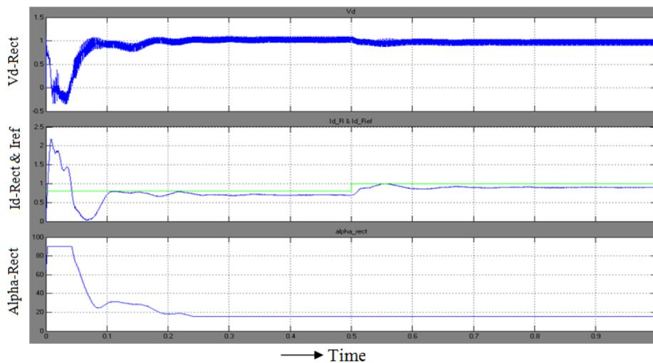
Fig 14. Rectifier side DC Voltage, DC Current and firing angle order with ANN
