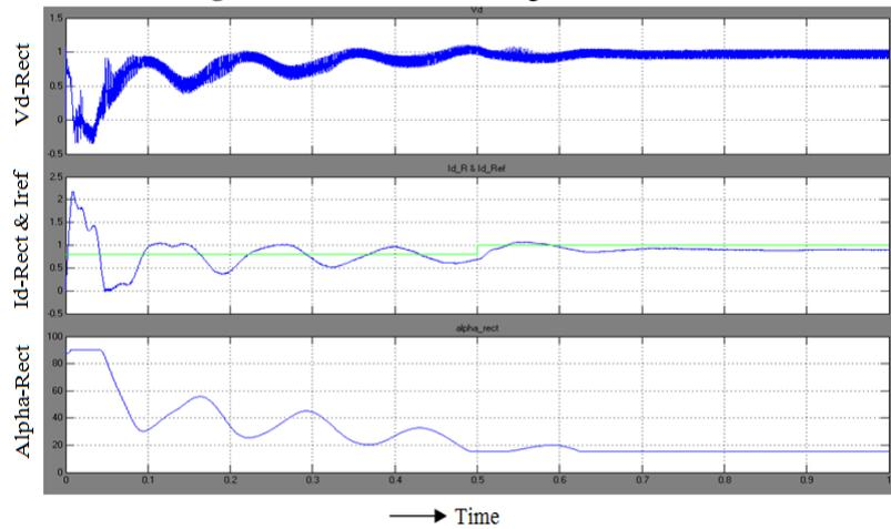
**Fig 8.** Rectifier side DC Voltage, DC Current and firing angle order with PI
