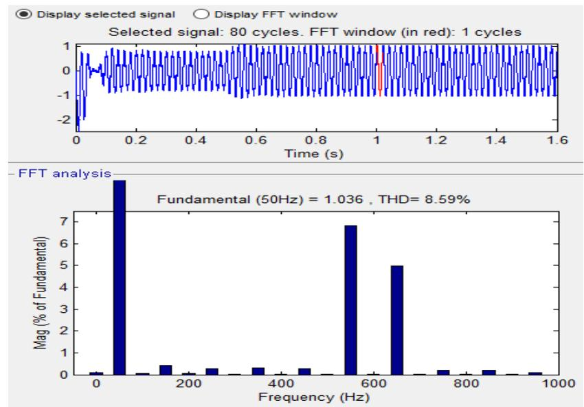
Fig.19 THD Analysis for Inverter Current using ANN controller
