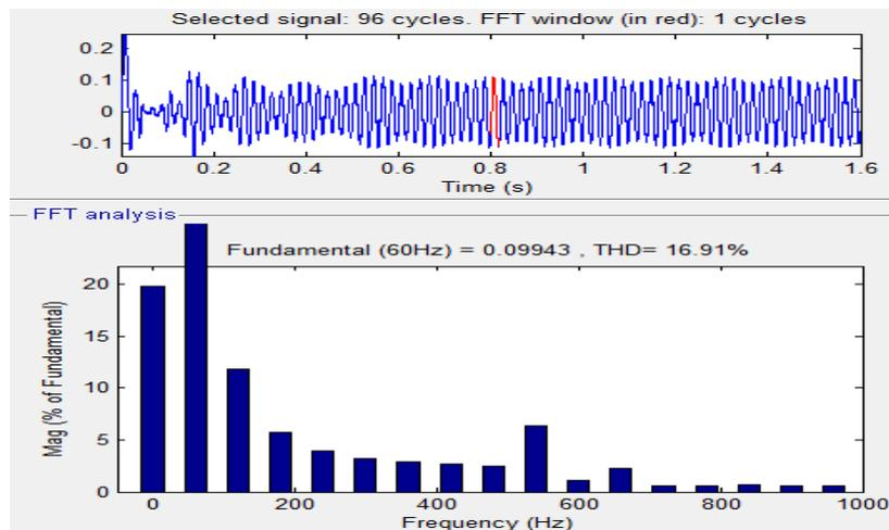
**Fig.16** THD for Rectifier current with PI controller
