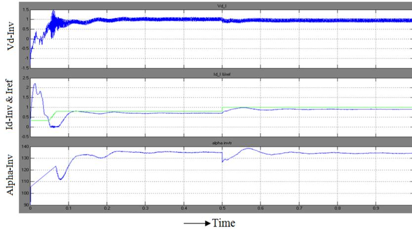
**Fig 15.** Inverter side DC Voltage, DC Current and firing angle order with ANN
